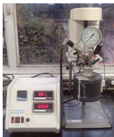
Figura 7: Reator Pressurizado (Parr Instruments, 4566 Mini Reactor)
