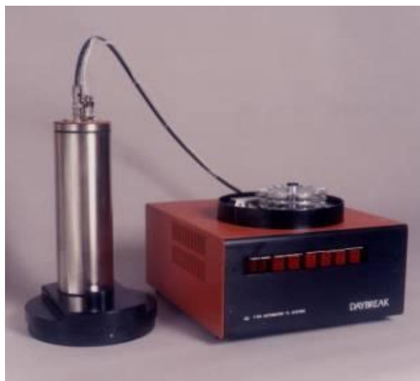
Figura 11: Daybreak 1100 Automatic TL/LOE System.
